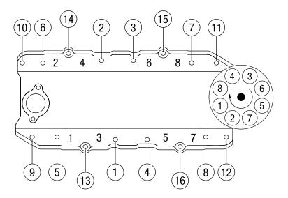
Figure 1 - Intake Manifold Bolt Tightening Sequence
