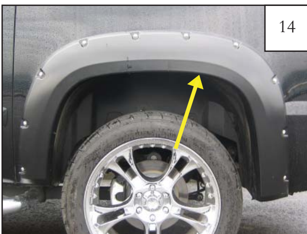
Install one supplied Retainer (RV1-P006) through rear corner hole in flare and into fender.
