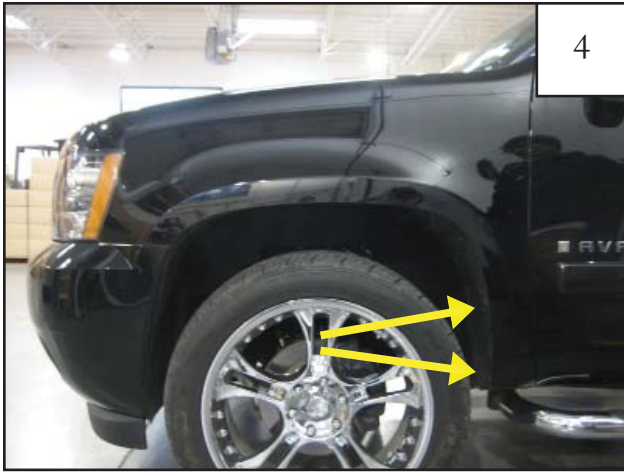
Using a 7mm socket, remove two factory screws. Retain screws for later use.
